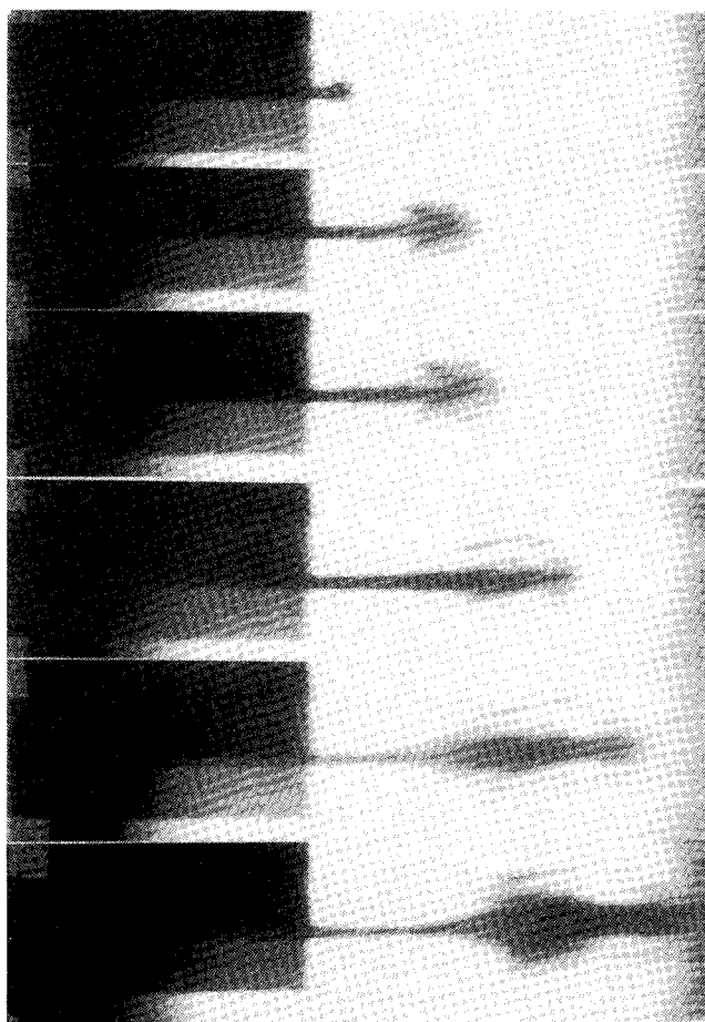
Fig. 9 Evolution of a plane free liquid jet using the x-ray radiography system.
